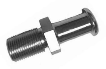
Designed as a companion part for use with single rotor latches that requires a 10mm (.394") diameter striker pin and compliance to FMVSS 206 (ECE R11).
